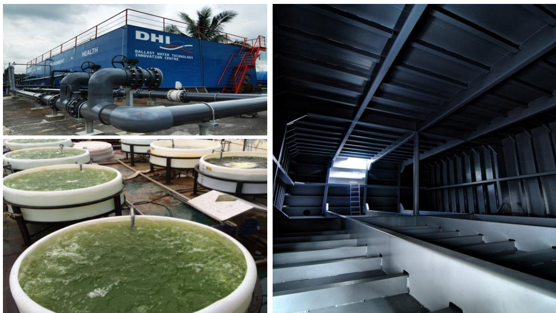
Fig. 3. Top left: the DHI ballast water technology and innovation centre in Singapore, bottom left: cultures of standard test organisms ( Tetraselmis sp.); right: inside a 250 m 3 retention tank used for mimicking ballast water transported during a ship's voyage.
