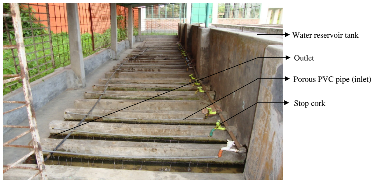
Fig. 1. The culvert system.
